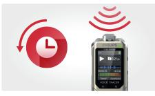
The pre-recording function allows you to record the last five seconds before you press the record key. The device switches into a standby mode and records a five-second loop without saving it. Press the record key to save the five-second loop. This feature allows you to spontaneously record important parts of a conversation.
